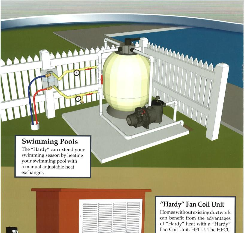
Homes without existing ductwork can benefit from the advantages of "Hardy" heat with a "Hardy" Fan Coil Unit, HFCU. The HFCU is an attractive finished furniture cabinet containing a hot water coil and fan. Water is circulated from the "Hardy" heater to the HFCU which is located inside your home. The fan inside the HFCU forces hot air across the water coil and heats your home, while a thermostat mounted on an electrical outlet adjacent to your HFCU regulates the temperature.
