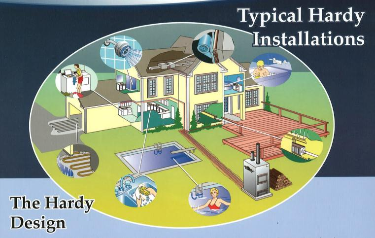
The "Hardy" Outside Woodburning Heater is designed to be located between 10 feet and 100 feet from your home, next to your firewood storage for convenient loading. This removes the fire danger from your home and keeps wood trash, smoke, and ashes out of your home. The "Hardy" heater is constructed of stainless steel to provide the best heat transfer, which is three times greater than 3/8" carbon steel.
